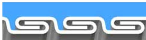
Interlocked Design 1-1/2" through 3" with no bonding wire
